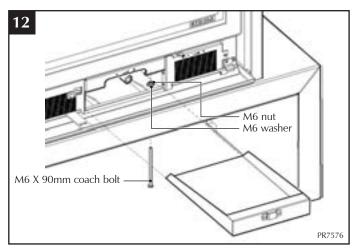
12 Remove ash pan and insert the two coach bolts in the front holes, fixing with the nuts and washers provided.
